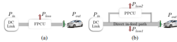
Fig. 2: Representative power flow diagram. (a) Full power charging unit. (b) Series-pass partial power charging unit.
